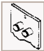
Threaded connection with alloy nozzle
