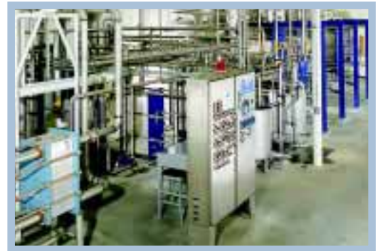
A five-effect SIGMASTAR® Plate Evaporator installation.
