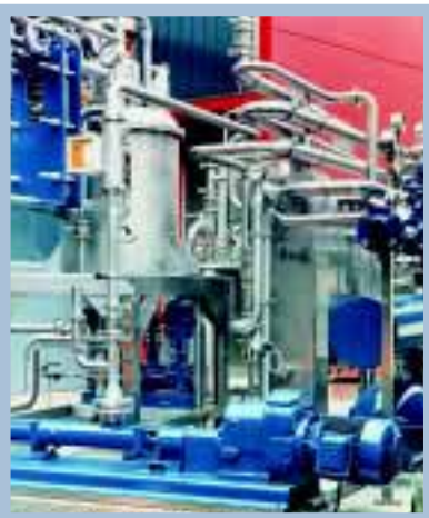
A pasteurization system with product deaeration.
