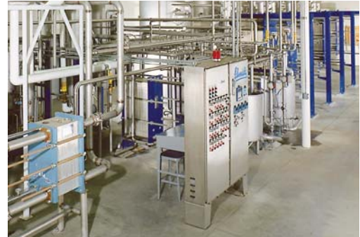
A five-effect SIGMASTAR® Plate Evaporator installation
