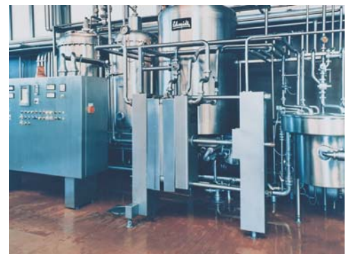
SIGMATHERM Pasteurization plant with deaeration
