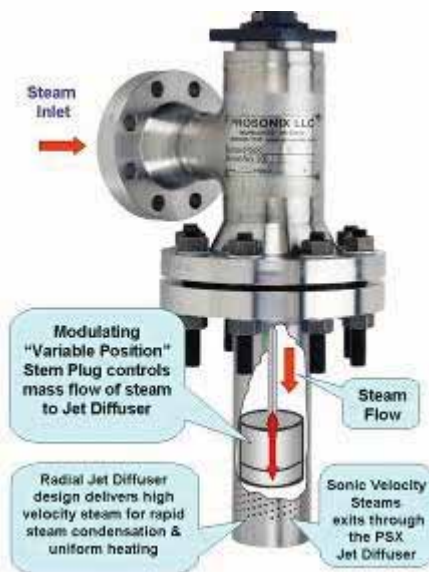
PSX Jet Diffuser Internal View
