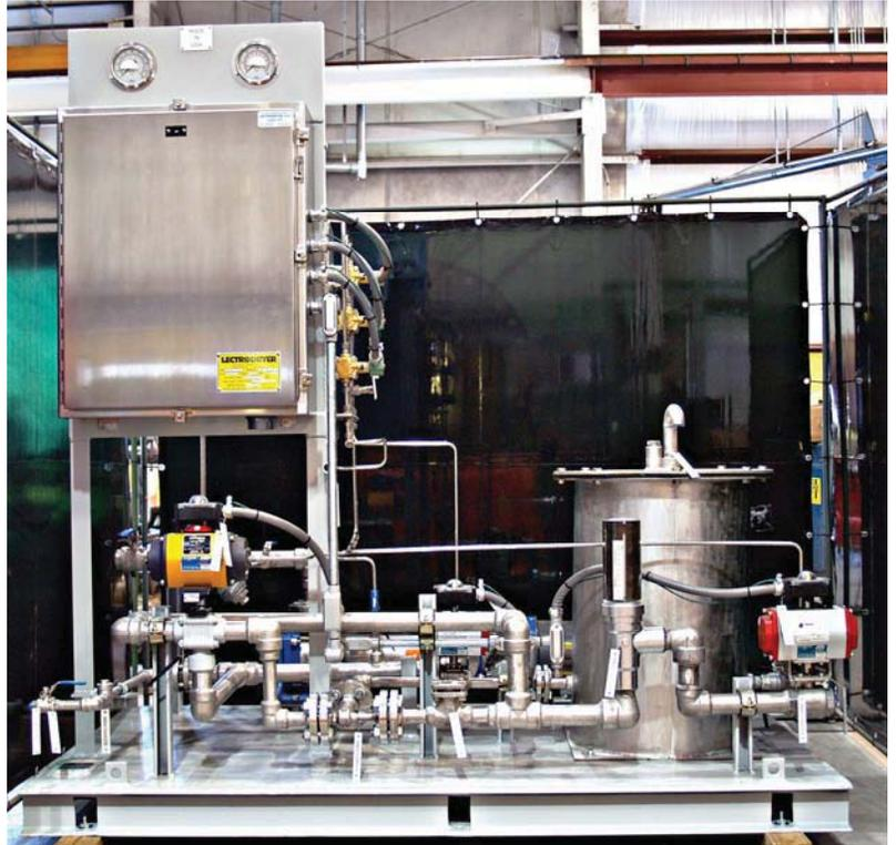
All 3 systems are designed to perform online and offline compressor water washing by supplying de-mineralized water or water and detergent to the gas turbines spray nozzles internal to the compressor plenum. Online compressor washing is utilized to prevent build up of heavy deposits on the compressor blades. Offline compressor washing is performed to eliminate heavier, more difficult accumulation.
